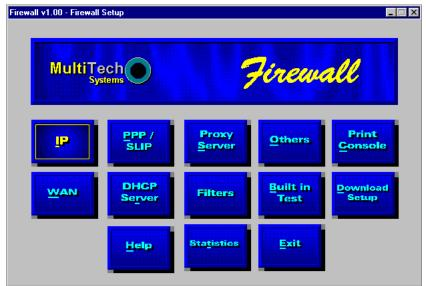
The **Firewall Setup** menu consists of 13 buttons which allow you to display and change the protocol stacks, define the output of the ProxyServer, perform network management functions, test the communications link, print messages received from the target ProxyServer, and download setup information to the ProxyServer.
